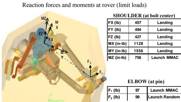
FIGURE 1: LOADS ANALYSIS- REACTION FORCES
